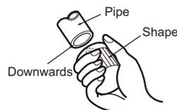
**C: Put on suitable insulating pipe**
