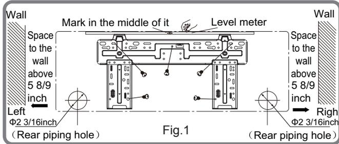
(2) Open a piping hole with the diameter of Φ2 3/16inch on the selected outlet pipe position. In order to drain smoothly, slant the piping hole on the wall slightly downward to the outdoor side with the gradient of 5-10°. (As show in Fig.2)
