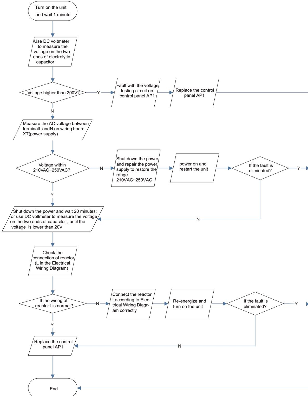
**(2) IPM protection, phase current overcurrent (the control board as below indicates the control board of outdoor unit) H5/P5**
