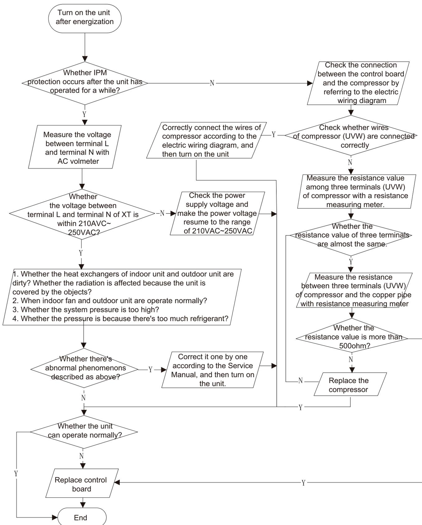
**(4) Start-up failure (following AP1 for outdoor unit control board)**
