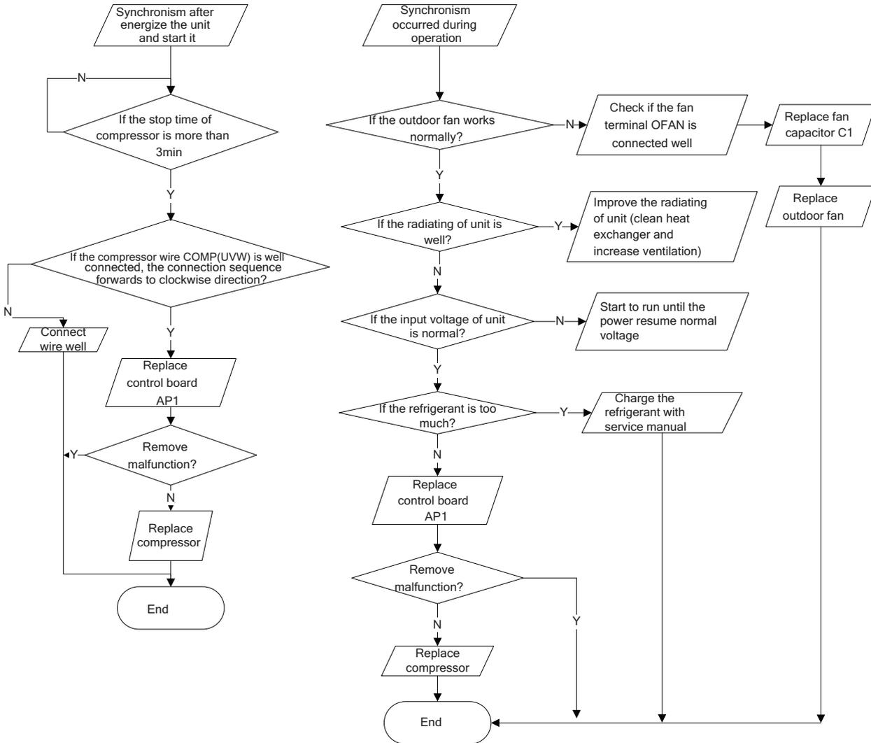
7.Diagnosis for overload and discharge malfunction (AP1 below is control board of outdoor unit)
