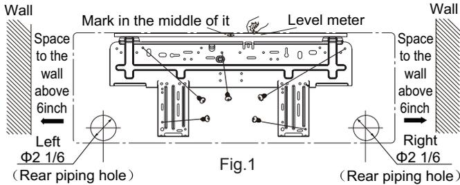
(2) Open a piping hole with the diameter of 2 1/6inch on the selected outlet pipe position. In order to drain smoothly, slant the piping hole on the wall slightly downward to the outdoor side with the gradient of 5-10°. (As show in Fig.2)
