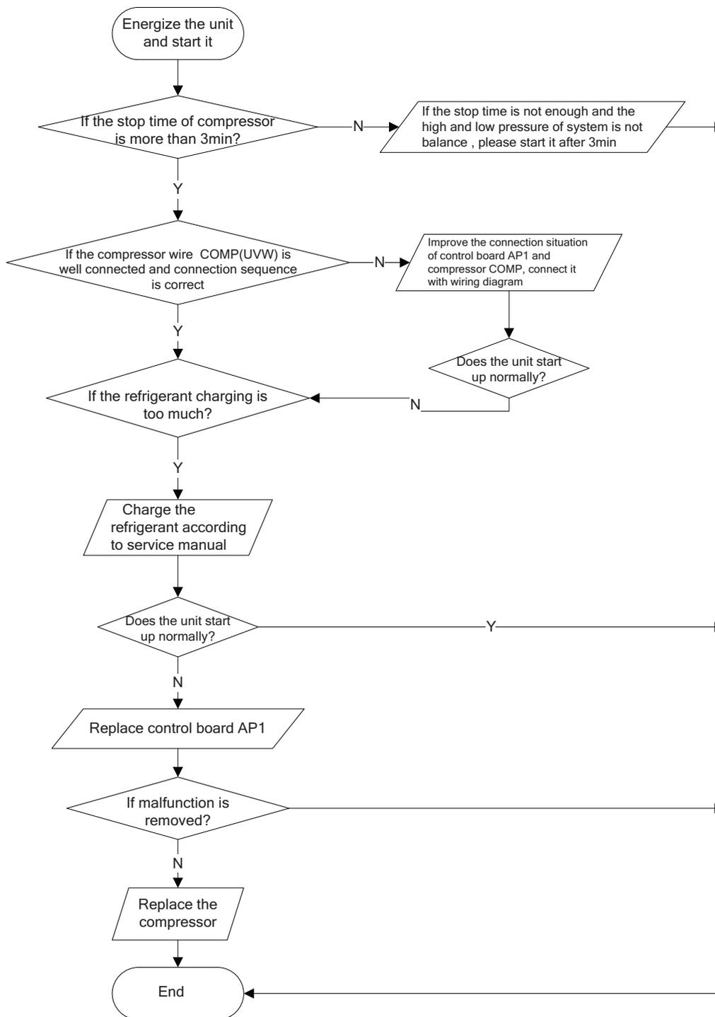
6. Diagnosis for compressor synchronism (AP1 below is control board of outdoor unit)
