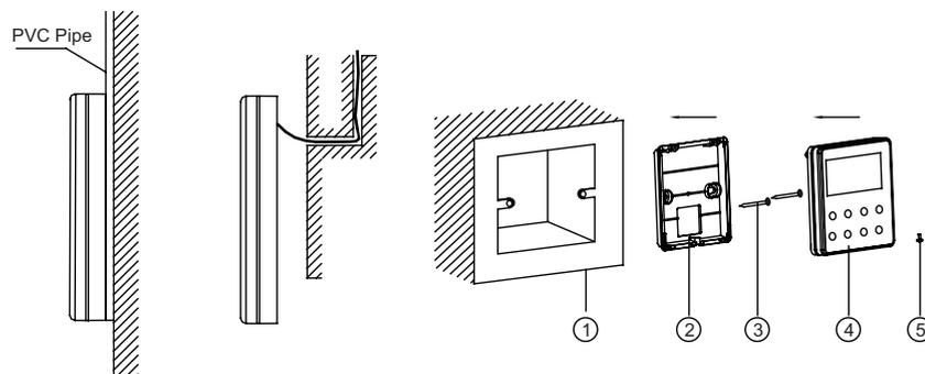
Fig.1.1 Accessories for the Installation of the Wired Controller
